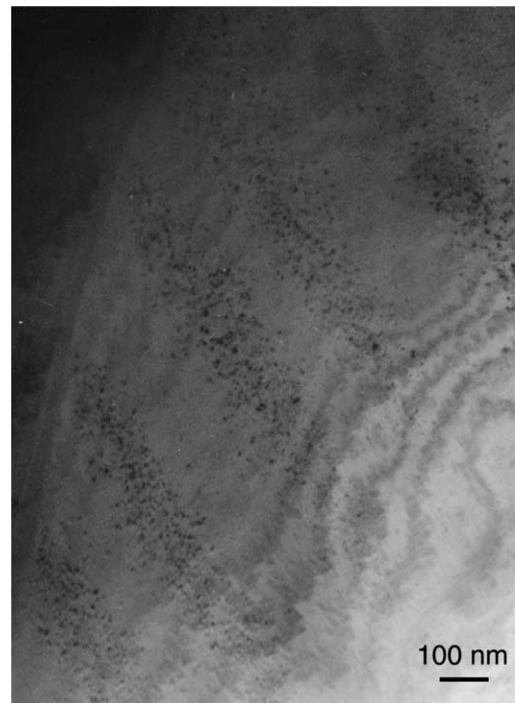
Fig. 8. Electron irradiated CVD-W at 573 K for 3 min (5 dpa).
